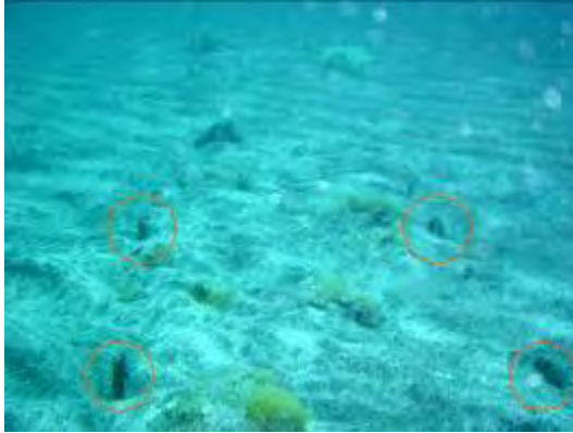
Fig. 10 Buried EMITE units, the lifting clamps are still visible
